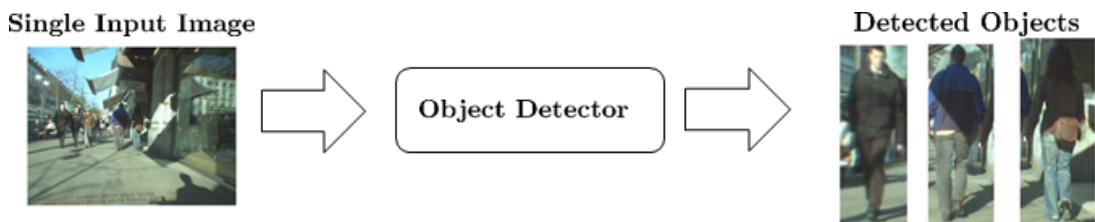
Figure 1.1: An illustration of a pedestrian detection system. It takes a single image as input and provides a list of all pedestrians.
