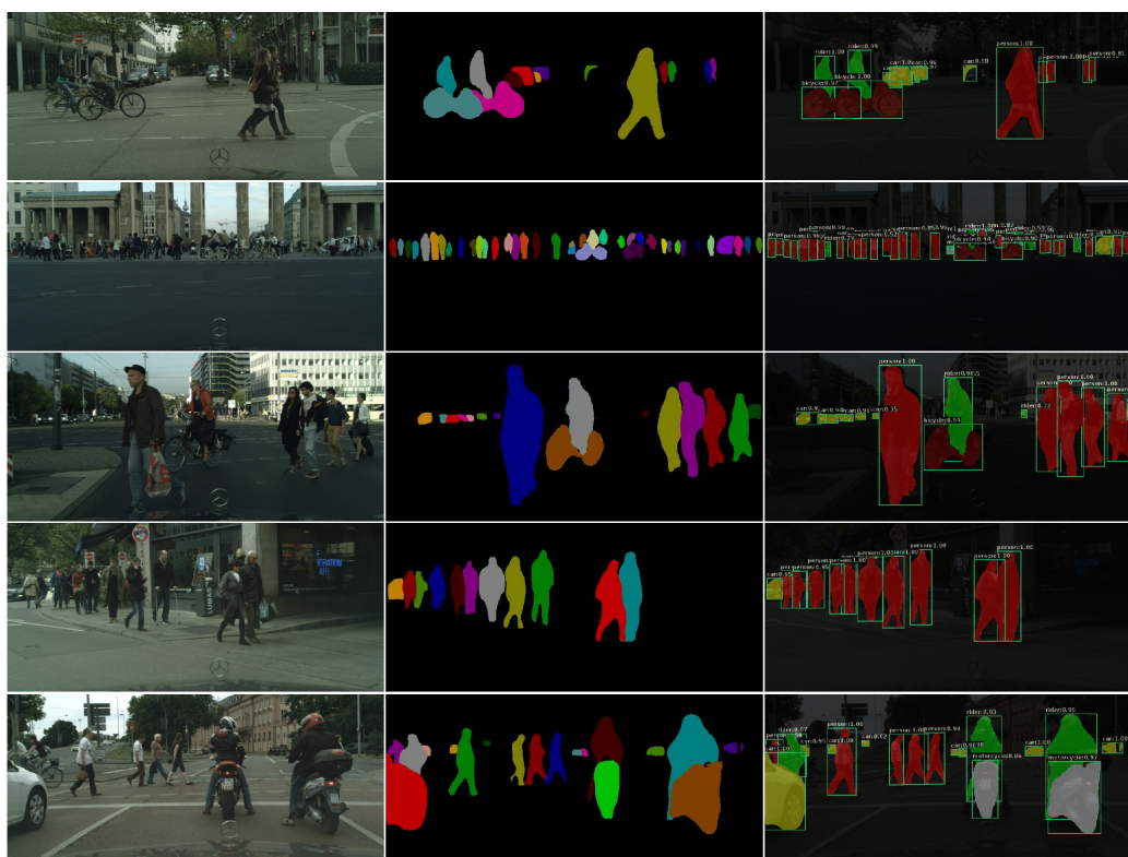
Figure 6.4: Qualitative results on Cityscapes From left to right, we show the input image, our instance level segmentations and the segmentations projected onto the image with class labels. Note that our segmentations are accurate despite the presence of many instances.
