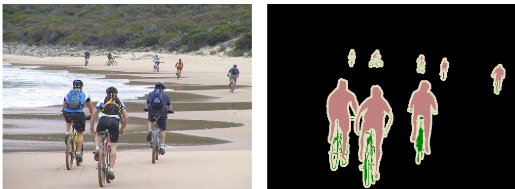
Figure 1.4: An illustration of a semantic segmentation. Left: An image from Pascal VOC 2012 [Everingham et al.], and Right: Ground-truth pixel-wise labeling.
