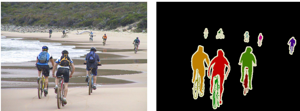
Figure 1.5: An illustration of semantic instance segmentation. Left: An image from Pascal VOC 2012 [Everingham et al.]. Right: Ground-truth pixel-wise instance semantic labeling.
